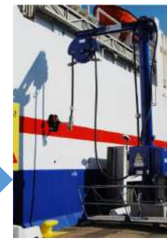
吊机式对接 Hoist type docking
