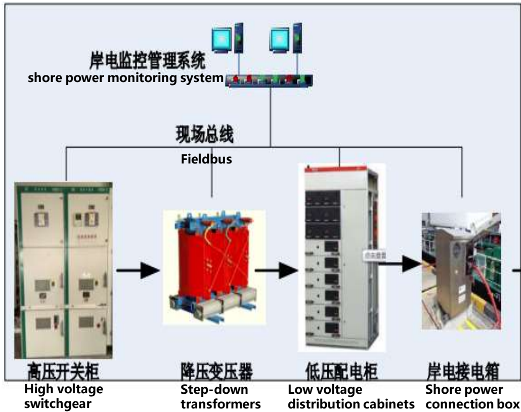
Shore Power Facilities
