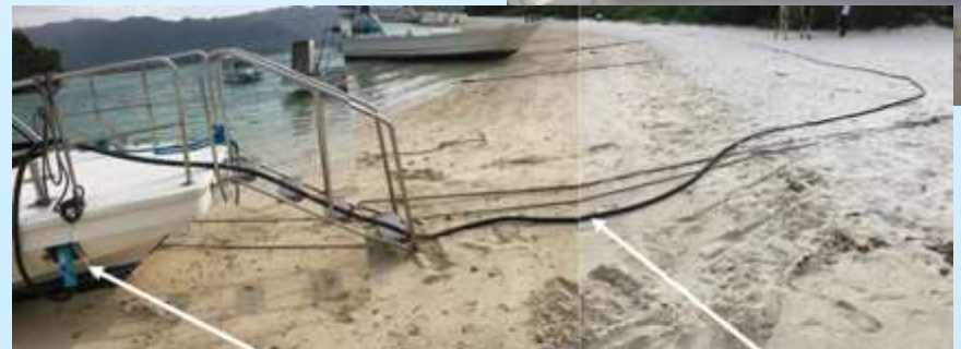
CHAdEMO with 60 m long cable
