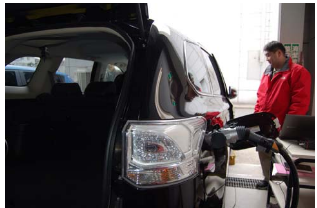
Connection test between a quick charger and a EV
