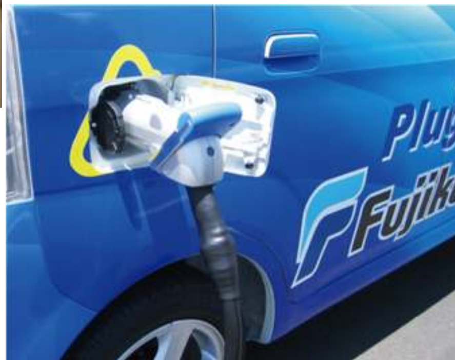
Connector plugged in EV
