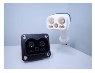
Temperature measurement of terminals with a cooling structure to cope with high currents, which was raised in ChaoJi TWS SWG 1, was carried out using an actual model with a current flow of 400 A. The results were reported and suggestions for ensuring safety were made.
